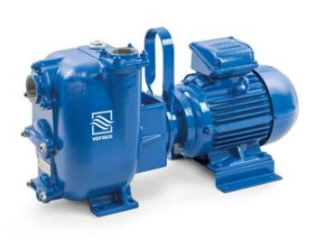
**Product Data** Suction port Threaded - 3" ISO 228 (BSP) Delivery port Threaded - 3" ISO 228 (BSP) Qmax 83 m<sup>3</sup>/h - 1383 l/min (365 USgpm) Hmax 30 m (98 ft) Solids handling 28 mm (1,1 ") Motor power 7,5 kW - 10 HP Motor type **IEC** standard Winding for inverters **Cast iron frame** Motor brand WEG W22 Premium Weight 131 ka
